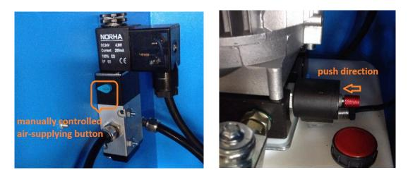
4. Close the unloading valve by pushing and turning clockwise the red core until you can hear the sound which implicate the valve is closed.
