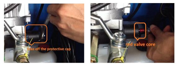
3. Push the blue air-supplying button and meanwhile push and turn anticlockwise the red valve core until sound which implicate the valve is open is heard. At this time, lifting platforms may lower.
