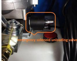
2. Take off the protective cap of the valve and see red the valve core.
